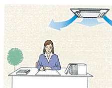
Draft-less air distribution can be performed by horizontal blow.
